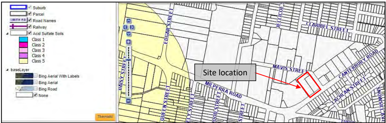
Figure 3 - The Site is determined to be no risk in regards to acid sulfate soil risk according to the Bankstown Local Environmental Plan 2015 (Screen shot adapted from http://gispublicviewer.bankstown.nsw.gov.au/bccgis/RestPublicApplication.aspx accessed on 21.12.2017)
